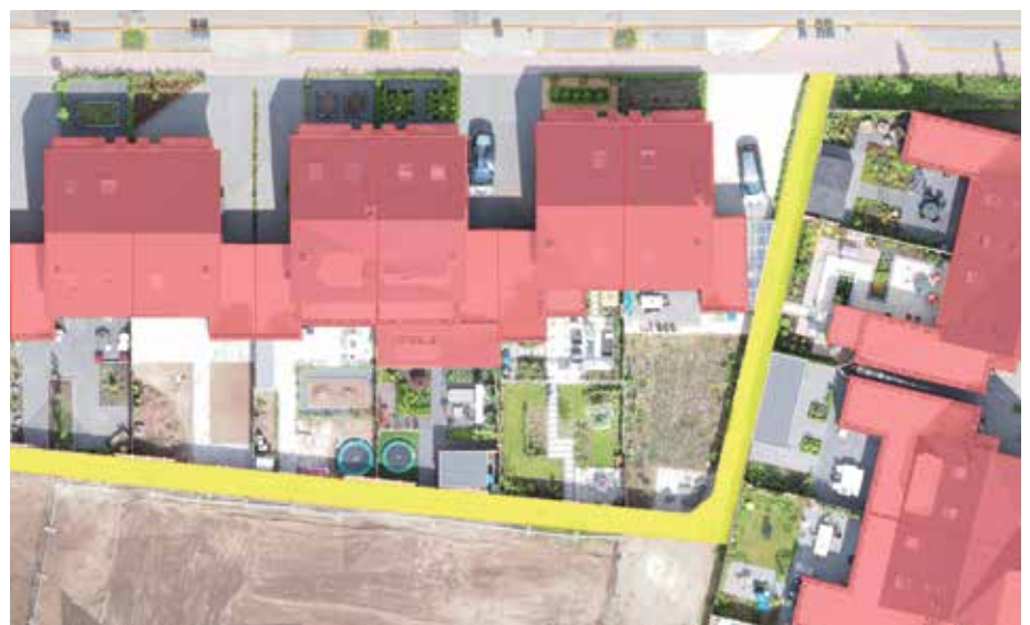
Result with stereo mapping and true orthophoto
