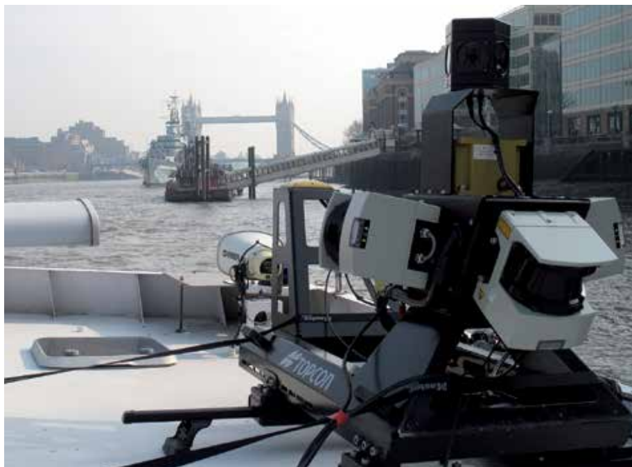
Topcon IP-S2 System – incorporating 360° Camera, IMU, GNSS and three Laser Scanners – installed on a River Thames survey vessel
