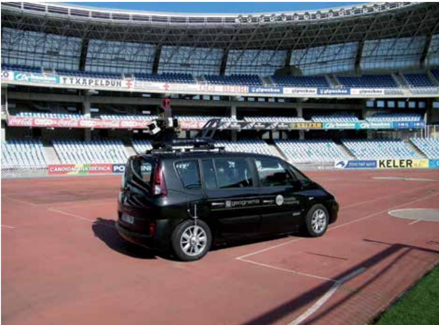
The Geograma mobile mapping vehicle, fitted with a Topcon IP-S2 system, scanners, panoramic camera, GNSS, IMU and odometer.
