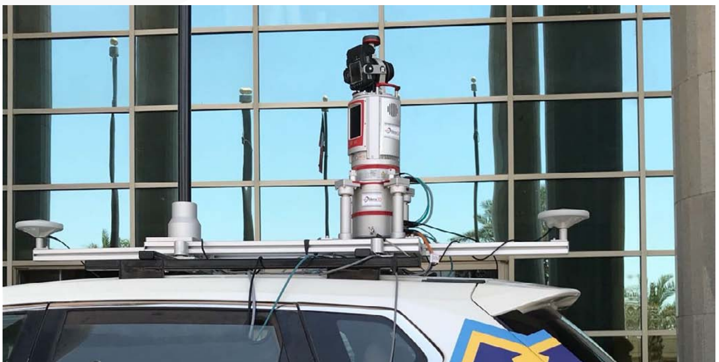
Mobile Mapping system mounted on vehicle (Source: PACI)
