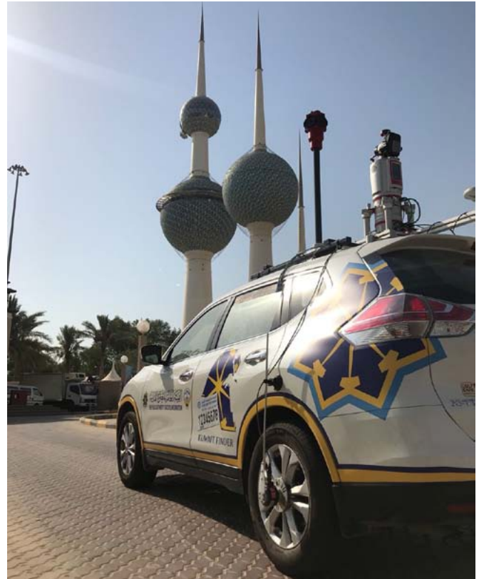
RIEGL VMZ VZ-400i Mobile Mapping system in Kuwait (Source: PACI)
