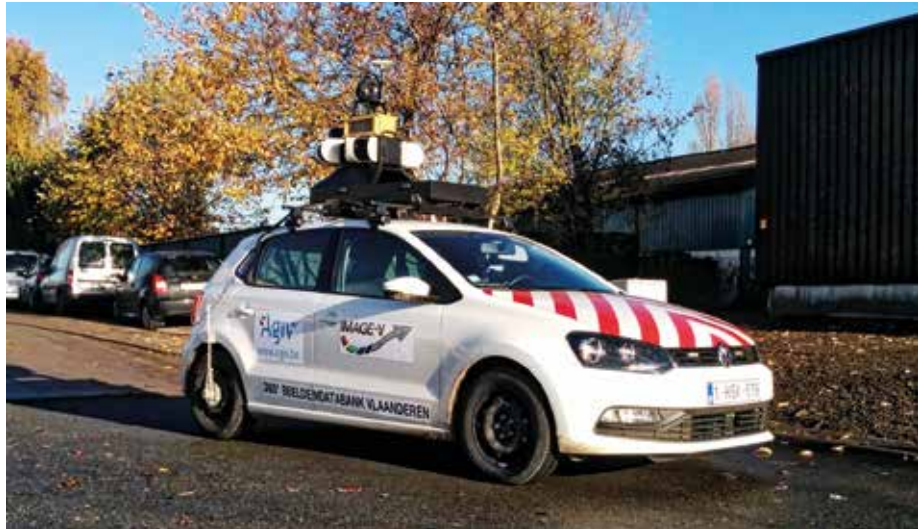
Image-V cars fully equipped with Topcon IP-S2 systems
