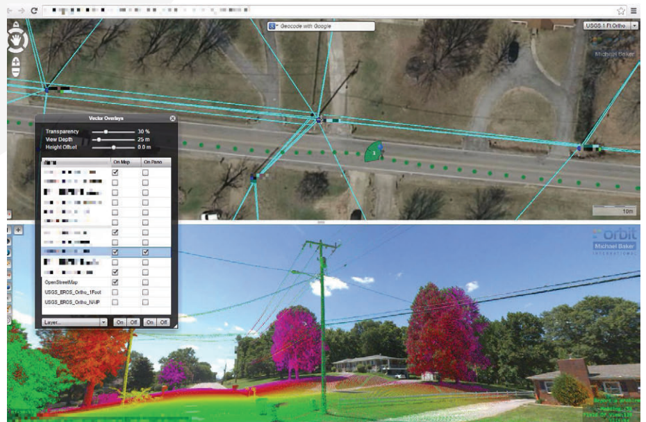
Figure 2: Analysing poles and equipment and catenary wire extraction to inventurise telco network shared with customer using Orbit MM Publisher.
