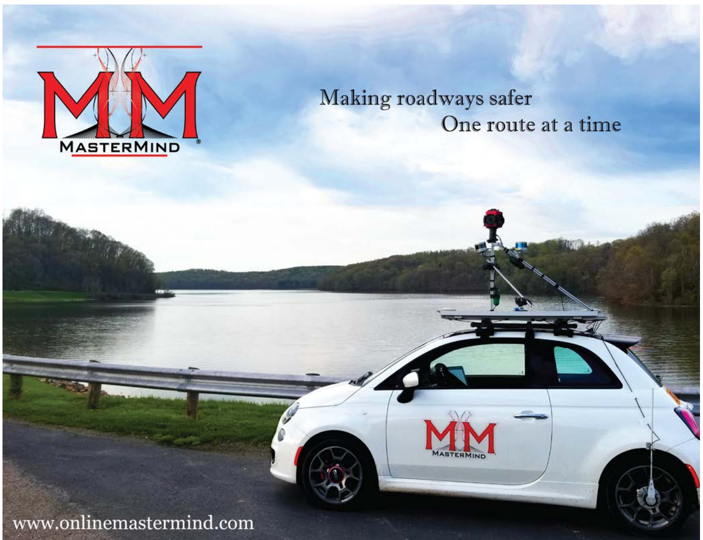
The MasterMind mobile mapping vehicle displaying the 360° camera, multiple LiDAR units, GPS antennas, the distance measuring instrument (DMI) and the solar panel.
