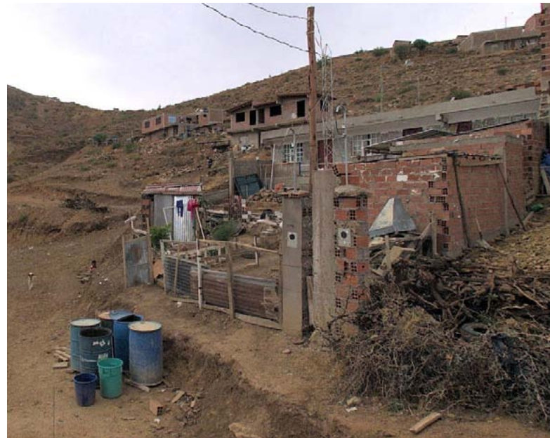
Area with very deficient urban infrastructure. The water barrels in front of the house are used to receive water from water trucks, two times per week
