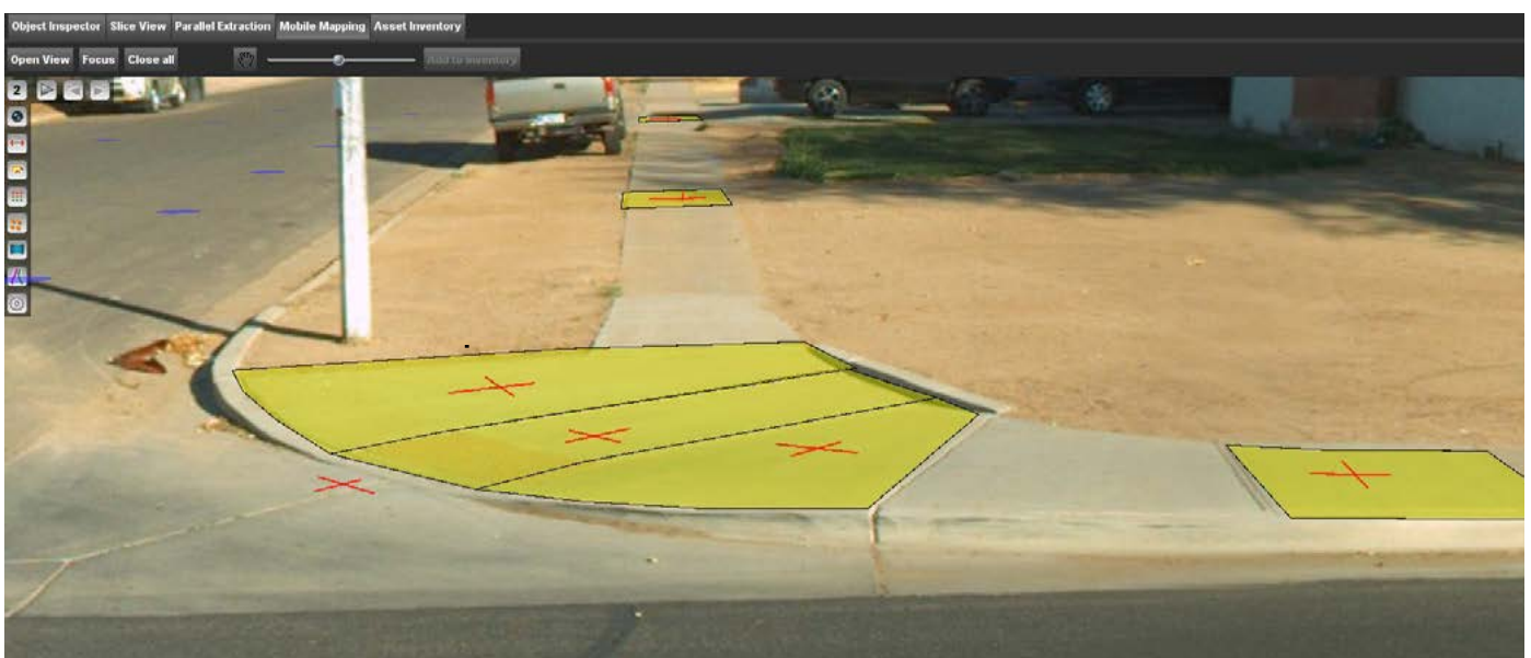
Ramp and sidewalk features with running slope and cross slope lines
